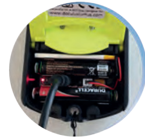
LI Lithium-Ion Battery
